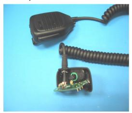
Ensure the crimp in positioned in the grommet. This will prevent the crimp from shorting out on the PCB.
