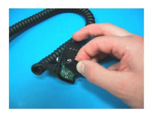
Step 3: De-solder the wires from the PCB: (not required for TOPA-AA-105)
