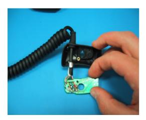
Step 12: Insert Green Locking Ring and Locking Lever into the Housing.
