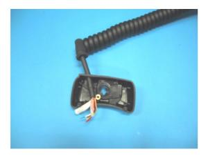
Step 9: Insert Cable and Grommet into the Tait Orca Housing:
