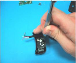
Step 5: Remove the Rubber Seal from around the D-Clip hole.
