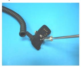
Step 2: Remove rubber PCB seal
