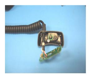
Step 13: Move the cable crimp into the cable grommet: (not required for TOPA-AA-105)
